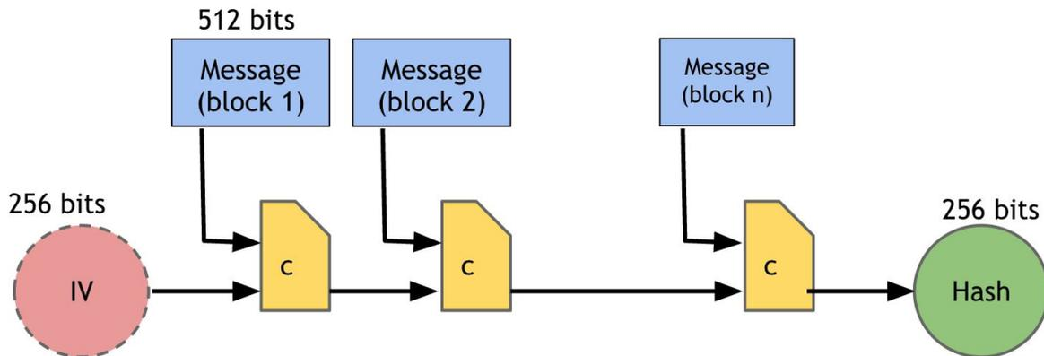
**Figure 1.3: SHA-256 Hash Function (simplified).** SHA-256 uses the Merkle-Damgard transform to turn a fixed-length collision-resistant compression function into a hash function that accepts arbitrary-length inputs. The input is “padded” so that its length is a multiple of 512 bits.
