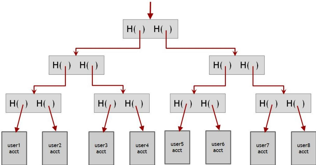
**Figure 4.5: Proof of liabilities.** The exchange publishes the root of a Merkle tree that contains all users at the leaves, including deposit amounts. Any user can request a proof of inclusion in the tree, and verify that the deposit sums are propagated correctly to the root of the tree.
