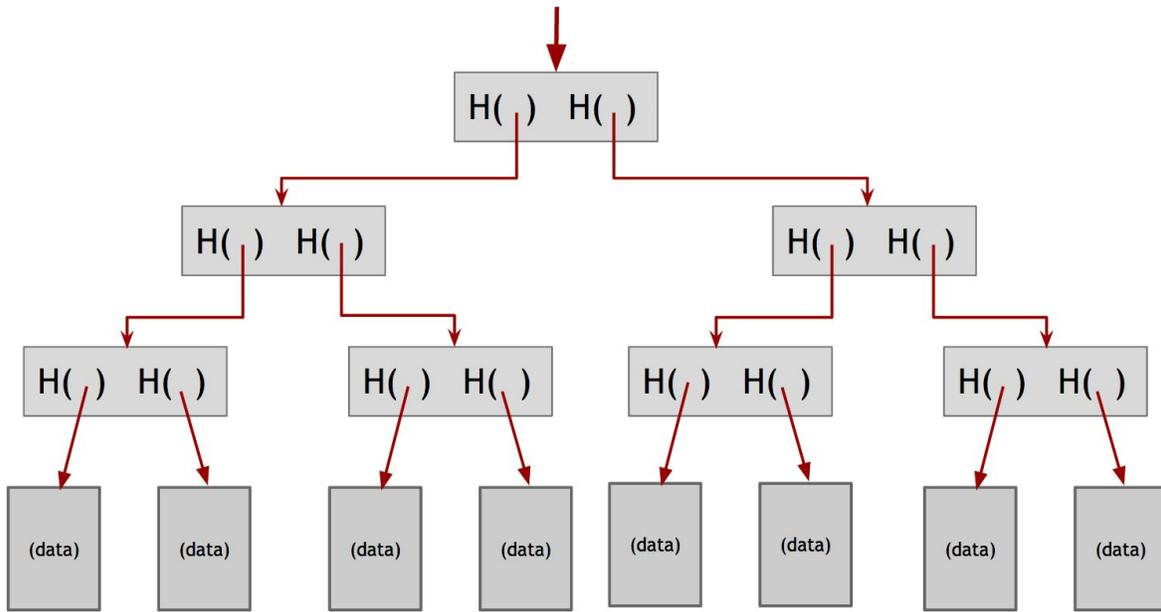
**Figure 1.7 Merkle tree.** In a Merkle tree, data blocks are grouped in pairs and the hash of each of these blocks is stored in a parent node. The parent nodes are in turn grouped in pairs and their hashes stored one level up the tree. This continues all the way up the tree until we reach the root node.
