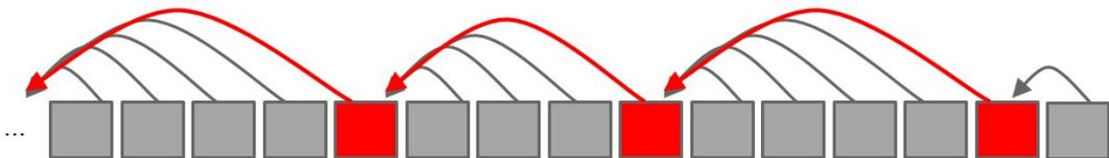
**Figure 10.7: a proof-of-work skiplist.** Blocks contain pointers both to the previous block and to the nearest block that satisfies  $hash < target / 4$ . The concept could be applied recursively, with a third level of pointers to blocks satisfying  $hash < target / 16$ , and so on.
