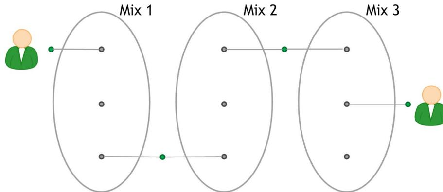
**Figure 6.8. Series of mixes.** We begin with a user who has a coin or input address that we assume the adversary has managed to link to them. The user sends the coin through various mixes, each time providing a freshly generated output address to the mix. Provided that at least one of these mixes destroys its records of the input to output address mapping, and there are no side-channel leaks of information, an adversary won't be able to link the user's original coin to their final one.
