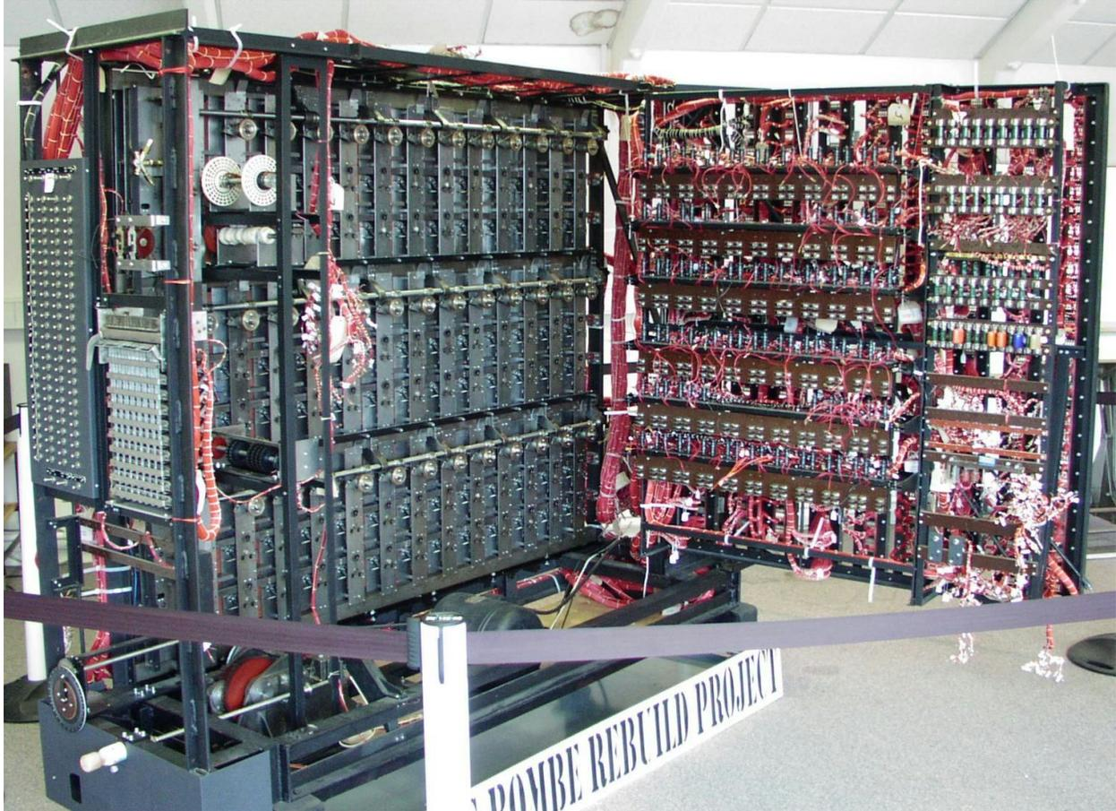
**Figure 10.8: A rebuilt Bombe machine located at the Bletchley Park museum.** The Bombe was a special-purpose computer designed by Alan Turing to crack German Enigma ciphers. Will Ethereum do to application-specific altcoins what the general-purpose computer did to Bombe-like contraptions?
