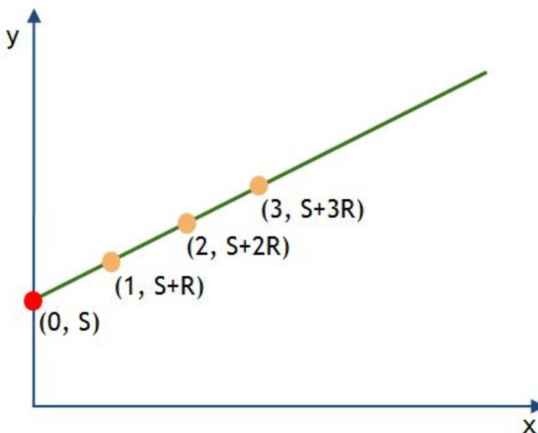
**Figure 4.4: Geometric illustration of 2-out-of- $N$  secret sharing.**  $S$  represents the secret, encoded as a (large) integer. The green line has a slope chosen at random. The orange points (specifically, their Y-coordinates  $S+R$ ,  $S+2R$ , ...) correspond to shares. Any two orange points are sufficient to reconstruct the red point, and hence the secret. All arithmetic is done modulo a large prime number.
