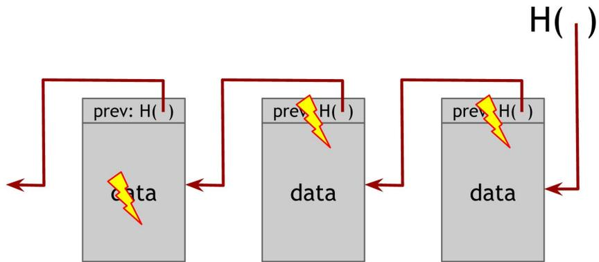
**Figure 1.6 Tamper-evident log.** If an adversary modifies data anywhere in the block chain, it will result in the hash pointer in the following block being incorrect. If we store the head of the list, then even if the adversary modifies all of the pointers to be consistent with the modified data, the head pointer will be incorrect, and we will detect the tampering.
