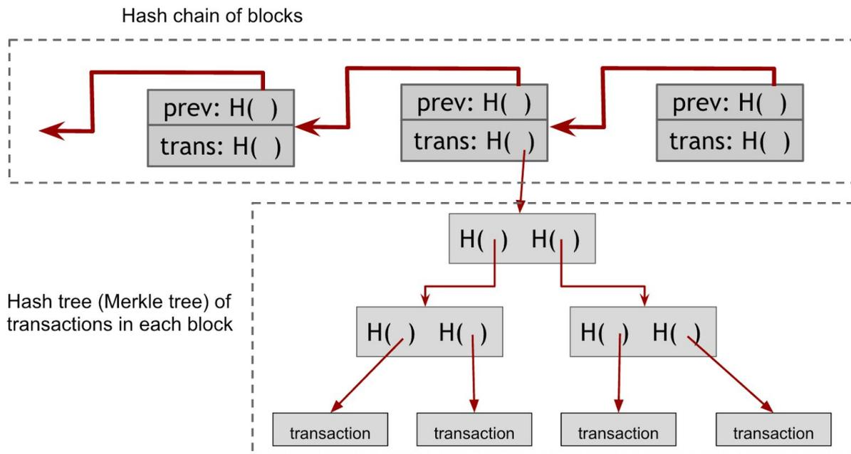
**Figure 3.8.** The Bitcoin block chain contains two different hash structures. The first is a hash chain of blocks that links the different blocks to one another. The second is internal to each block and is a Merkle Tree of transactions within the blocks.
