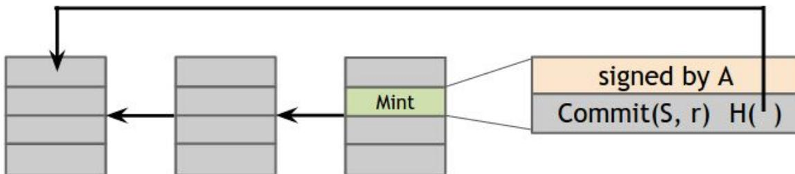
**Figure 6.12: Putting a zerocoin on the block chain.** To put a zerocoin on the blockchain, you create a special 'mint' transaction whose output 'address' is the cryptographic commitment of the zerocoin's serial number. The input of the mint transaction is a basecoin, which has now been spent in creating the zerocoin. The transaction does *not* reveal the serial number.
