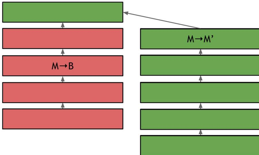
**Figure 5.15 Forking attack.** A malicious miner sends a transaction to Bob and receives some good or service in exchange for it. The miner then forks the block chain to create a longer branch containing a conflicting transaction. The payment to Bob will be invalid in this new consensus chain.
