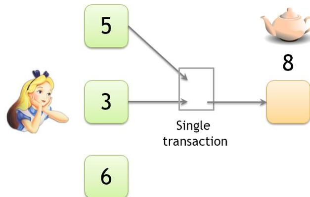
**Figure 6.2 :** To pay for the teapot, Alice has to create a single transaction having inputs that are at two different address. In doing so, Alice reveals that these two addresses are controlled by a single entity.
